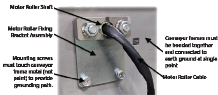
Image 14: MDR Mount to Conveyor Frame
