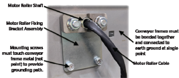
Image 12: MDR Mount to Conveyor Frame
