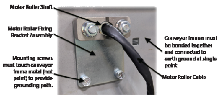
Image 14: MDR Mount to Conveyor Frame
