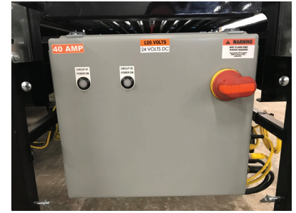
Figure 7: Power Panel with Disconnect Switch
